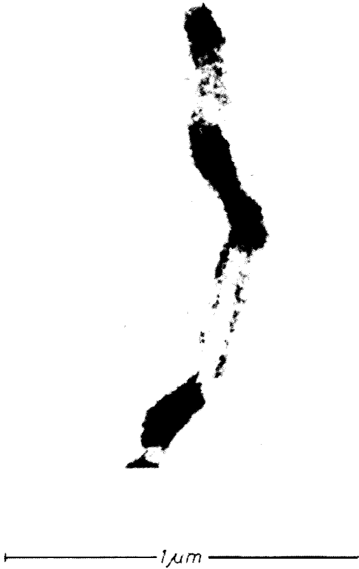
Fig. 9.: Iron Whisker ( U = 79 \text{ kW} , M_a = 3100 ) (Beischer, D., and Krause, F.: Naturwissenschaften 25, 825-829 (1937)).
