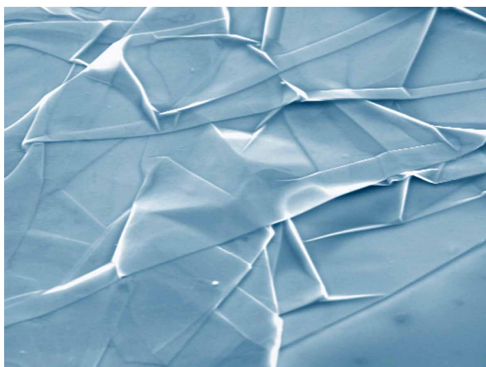
Figure 3. Like a silk sheet. Folded sheets of graphene on a silicon plate. The image was made with a scanning electron microscope, magnified about 5 000 times.
