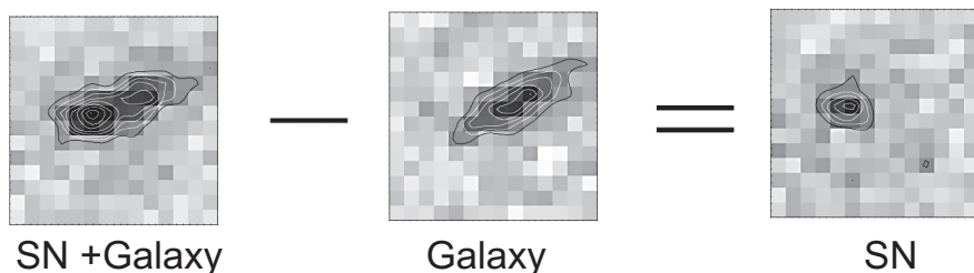
Figure 3. Example of digital image subtraction. From the CCD image of a supernova and its host galaxy, we subtract an image of the galaxy before the supernova appeared (or after it disappeared), leaving an image of just the supernova.
