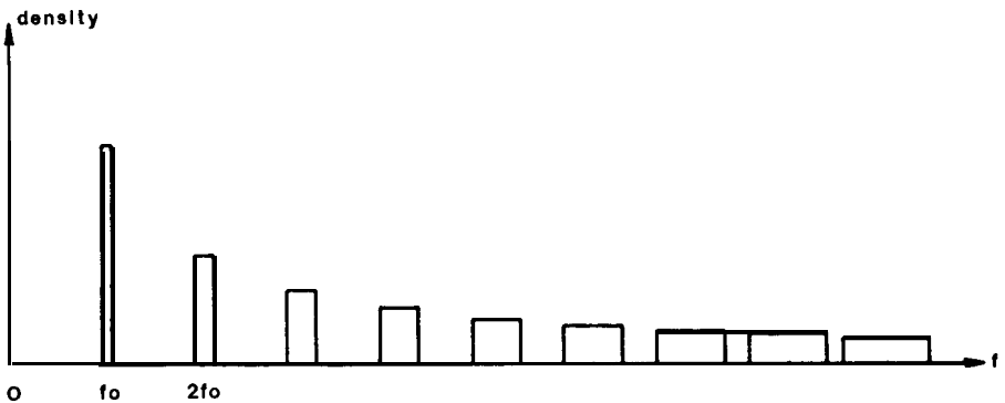
Fig. 5. Longitudinal Schottky bands originating from a large group of particles with slightly different revolution frequencies. At high frequencies the bands overlap.
