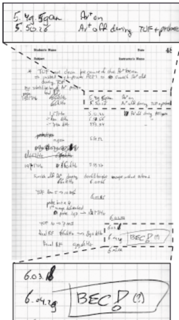
Figure 6. One page of the lab book during the night of September 29, 1995, when BEC was first observed at MIT. The handwriting is by Klaasjan van Druten. At 5:50 a.m., we had installed a new acousto-optical modulator to switch-off the optical plug (Ar ion laser beam). Fifteen minutes later, we had the first definitive evidence for BEC in sodium.
