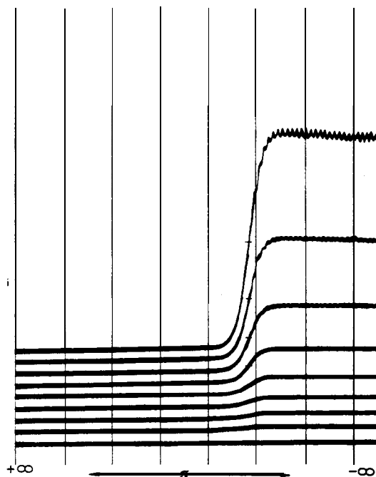
Fig. 7. Constancy of the half-wave potential in solution of various concentrations of \text{CdCl}_2 .
