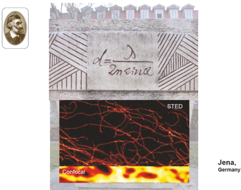
FIGURE 4. The diffraction resolution limit carved in stone (top: Memorial in honour of Ernst Abbe in Jena, Germany), and resolution increase in STED nanoscopy (middle) over confocal imaging (bottom).
