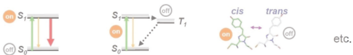
FIGURE 18. Paradigm shift in the use of the physical phenomenon by which features are discerned in a far-field fluorescence microscope: From focusing of light to using a molecular state transition, such as a transition between an “on” and an “off” state.
