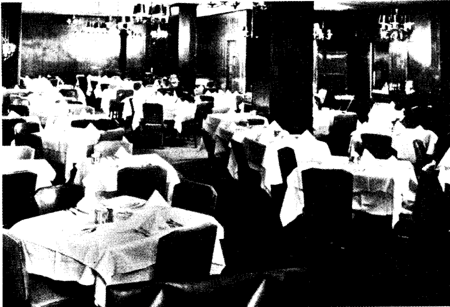
Fig. 13. Reconstruction of a Plane Transparency, Showing a Restaurant, from a Hologram taken with Diffused Illuminations (E. N. Leith and J. Upatnieks, 1964).
