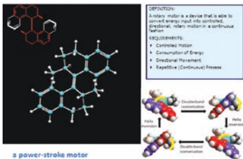
FIGURE 6. First generation light-driven rotary molecular motor and four stage rotary cycle.
