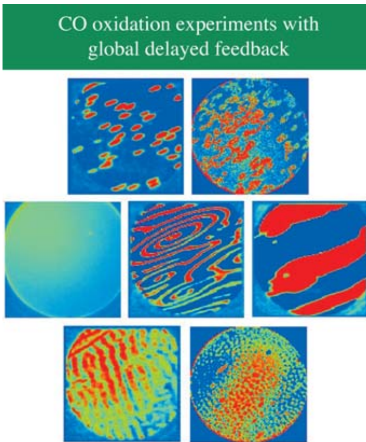
Figure 26. Transformation of a state of spiral turbulence into different other patterns by a feedback mechanism with different strength and delay of the feedback [51].
