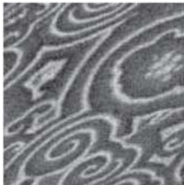
Figure 25. PEEM image from a Pt(110) surface in the state of chemical turbulence.
