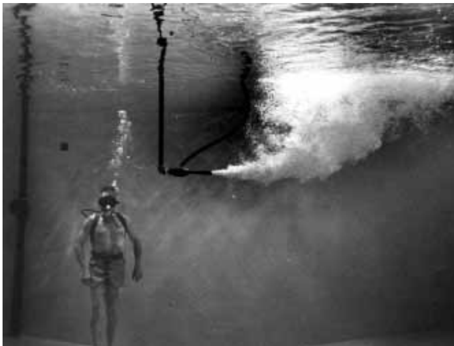
Figure 7. The eductors, which allowed efficient mixing of helium and perchloroethylene, are being tested here in the swimming pool at Brookhaven, using air and water. From the Brookhaven National Laboratory website, http://www.bnl.gov/bnlweb/raydavis/images/hires/11-755-04.jpg .
