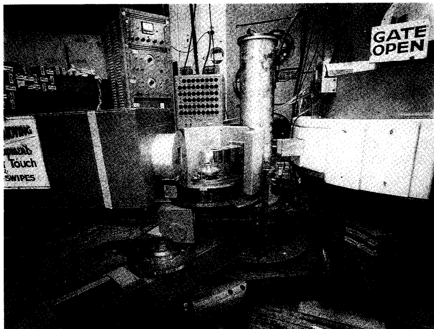
Fig. 9: Photograph (1959) of the original triple-axis spectrometer at the NRU reactor at Chalk River. The bank of 52 rotary switches, preset to go through an energy scan of up to 26 points, can be seen in the upper-centre. One of the three variables involved would traverse linearly through the domain of settings desired, while the other two advance nonlinearly according to the settings of the appropriate switches. (AECL photo)
