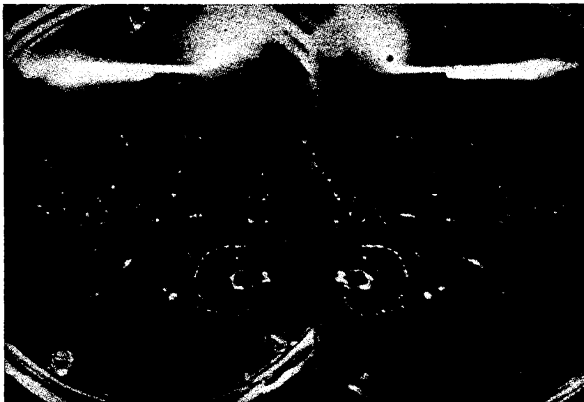
Fig. 4. Positrons produced in the disintegration of radioactive carbon of mass eleven units. (Magnetic field 780 gauss.) (The radioactive carbon was kindly supplied by Professor C. C. Lauritsen and his collaborators who prepared it by bombarding with deuterons a target containing boron.)
