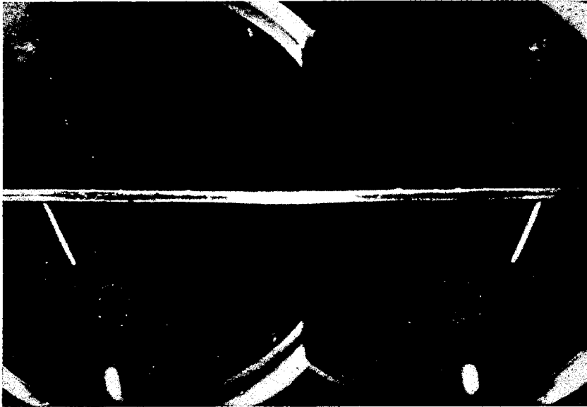
Fig. 11. A positron of 480 million electron-volts strikes a 0.35 cm lead plate. Below the plate three electrons appear having energies (in million electron-volts) respectively: positron 45, negatron 45, and positron 31. One of the tracks below the plate presumably represents the incident positron after passage through the plate, and the other two tracks a pair generated by the absorption of a photon generated in the plate. The energy lost in the plate by the incident positron is at least 435 million electron-volts and since the loss by ionization in a plate of this thickness should not be greater than 10 million electron-volts, the greater part of the energy lost by the positron in this instance must have appeared in the form of radiation. (Magnetic field 7,900 gauss.)
