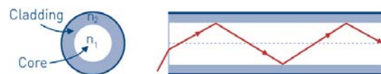
Fig. 1: Optical fiber. The refractive index of the core is slightly higher than that of the cladding. Typical dimensions are 10 or 50 micrometers for the core and 125 micrometers for the fiber. In addition, a protecting plastic “buffer” is placed around the fiber.
