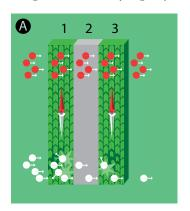
If the direction of the magnetization is the same in both magnetic layers the electrons with parallel spin (red) can pass through the entire system without scattering to any great extent. The total resistance of the system will therefore he small
