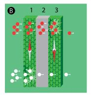
If the direction of magnetization in the two magnetic layers is opposed, all the electrons will have anti-parallel spin in one of the layers and will therefore scatter a great deal. As a result the total resistance is high.
